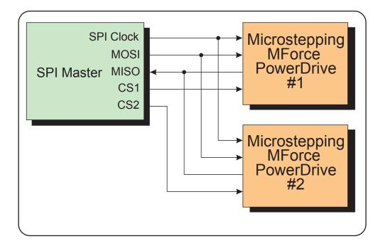
Figure 2.5.5: SPI Master with Multiple Microstepping MForce PowerDrives
